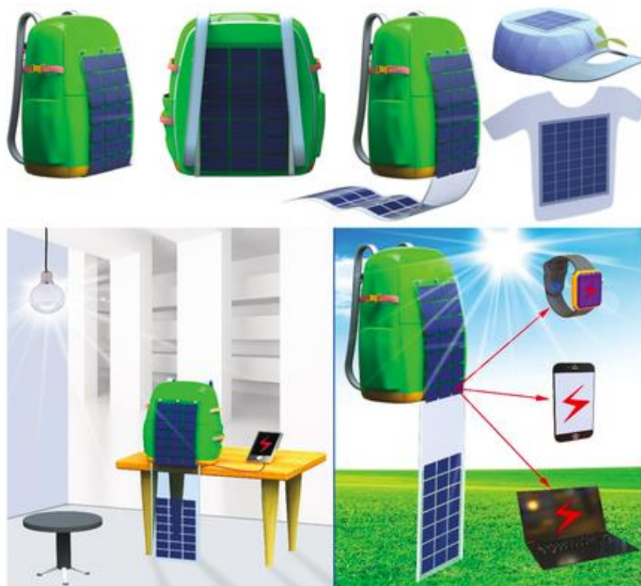
Figure 5 Solar cell on textiles for driven the portable device
