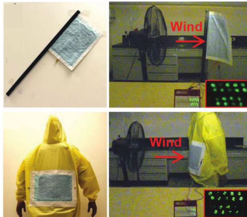
Figure 6 Wind energy harvesting through a flag and coat
