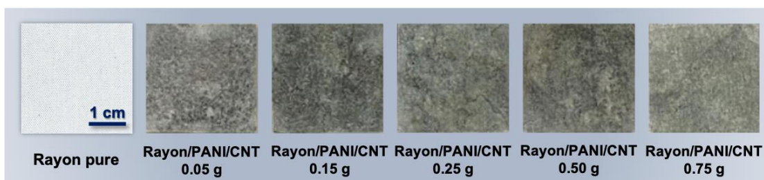
Figure 90 The digital images of pristine Rayon fabric and Rayon/PANI/CNT in various condition (0.05, 0.15, 0.25, 0.50 and 0.75 g)
