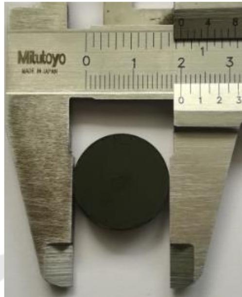
Figure 19 The pellets sample of  $\text{YBa}_4\text{Cu}_5\text{O}_y$
