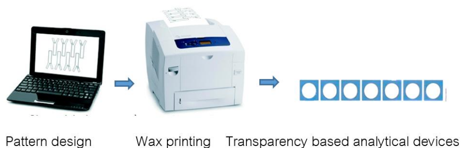
Figure 13 Fabrication process of pattern paper by wax printing.
