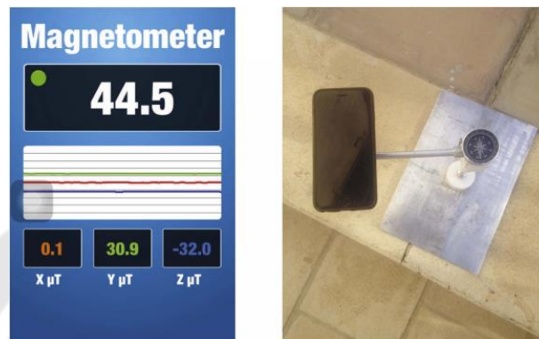
Figure 9. Screen of the Magnetometer application of the smartphone (left) and the experimental setup (right).
