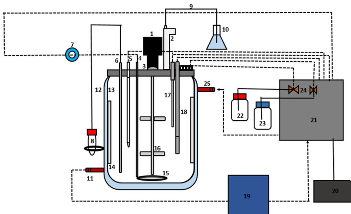
FIGURE 9 Schematic diagrams of 5-L stirrer bioreactor used throughout this study.
