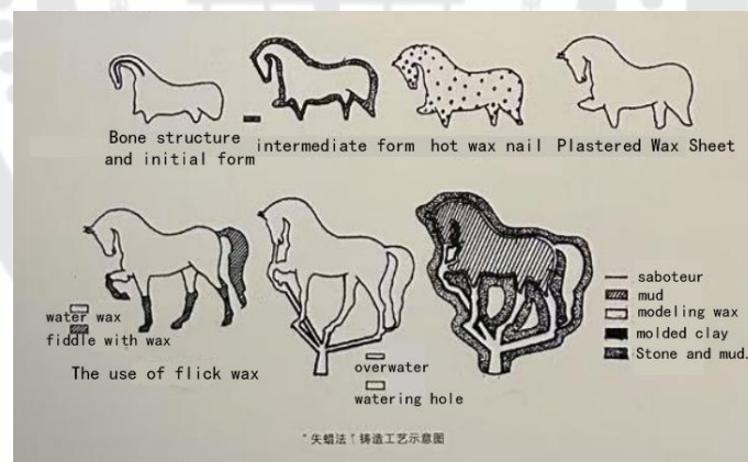
Figure 12 Lost wax casting process schematic
