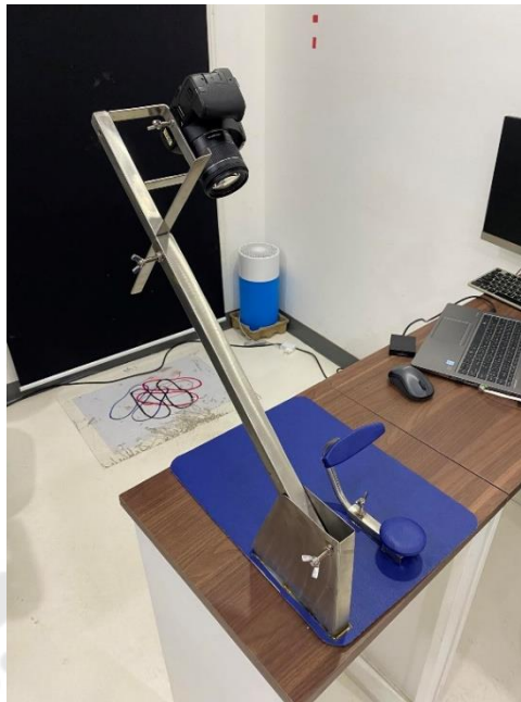
Figure 3.3 Stereotaxic instrument photographed from a 45-degree angle with an attached digital camera.
