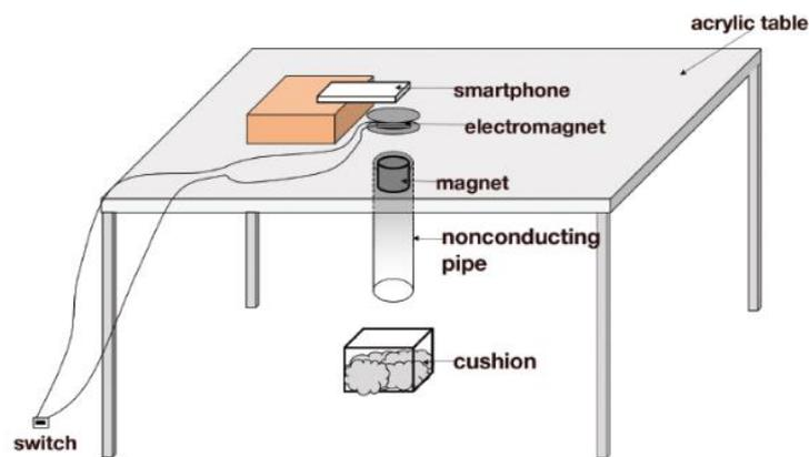
Figure 16 Table experimental setup to calculate acceleration due to gravity.
