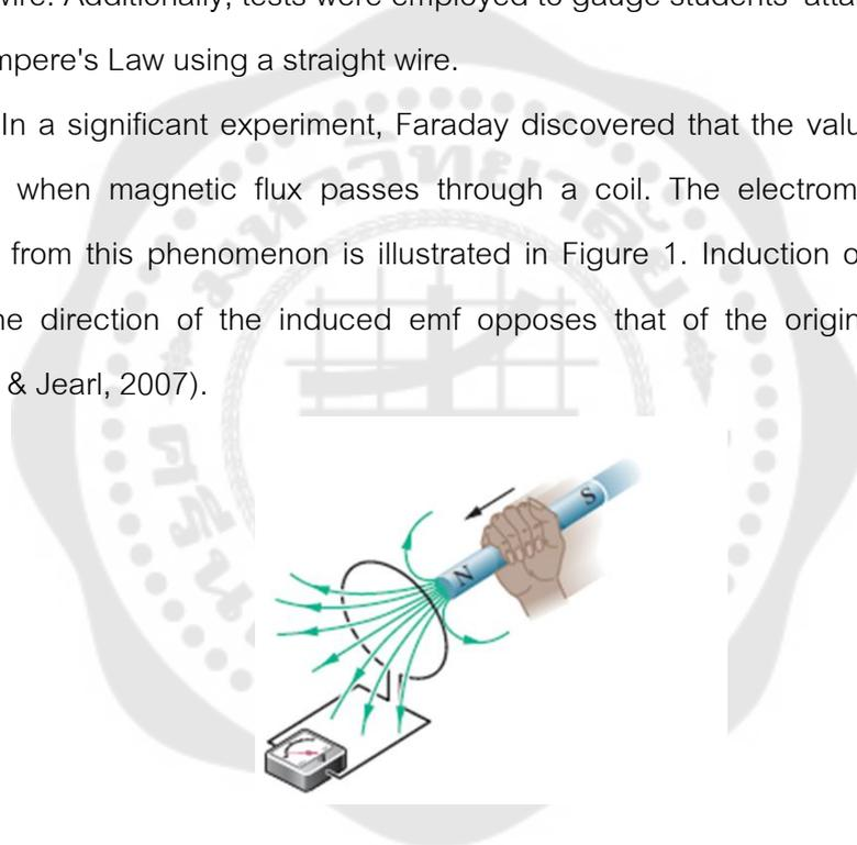
Figure 1 The electric current generated by the moving magnetic coil is detected by an ammeter.
