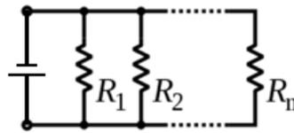
Figure 12 Connecting resistors in Parallel.
