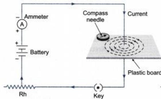
Figure 7 Observing magnetic region lines around an electrically conductive.
