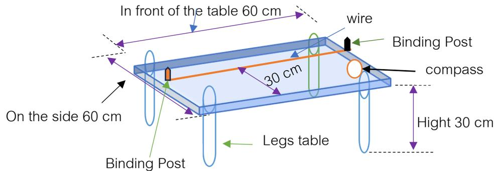
Figure 18 The acrylic table used for this experiment.
