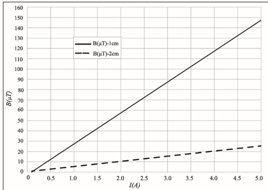
Figure 38 The relationship between the magnetic field and AC current.
