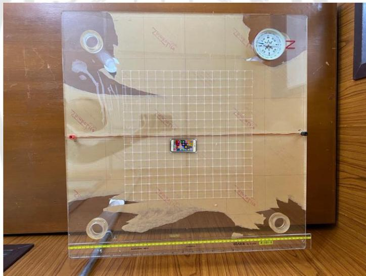
Figure 26 The smartphone was positioned 1–8 cm away from the wires.
