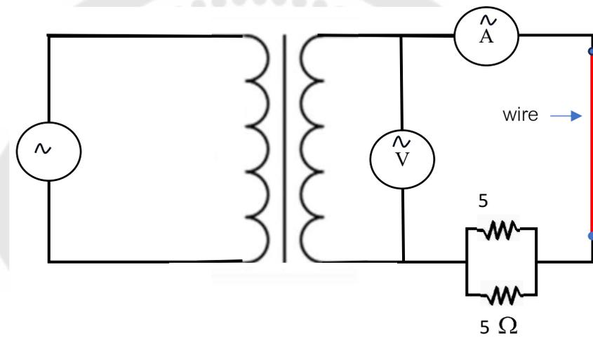
Figure 23 An electrical circuit including 2 resistors connected in parallel.
