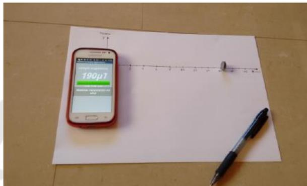
Figure 13 Experimental assembly in which you can perceive the small magnet and the smartphone.
