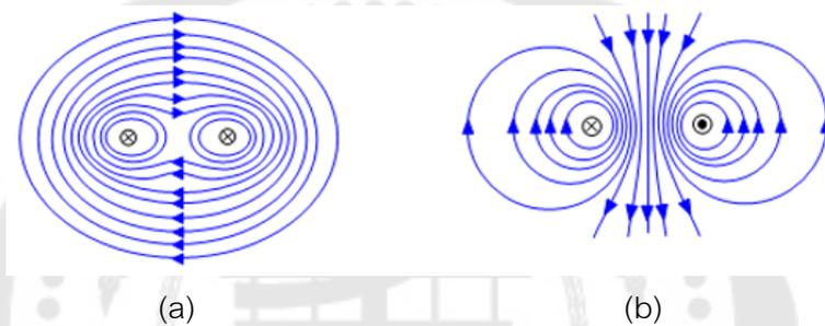
Figure 10 When two wires with current flowing in the same direction are placed close together.
