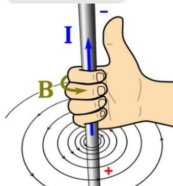
Figure 8 Right-hand rule of conductor.
