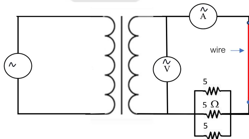
Figure 24 An electrical circuit with three resistors connected in parallel.
