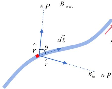
Figure 5 Magnetic field generated by electric current in conductors of any shape.
