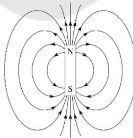
Figure 3 The flux line of magnetic field from magnet.
