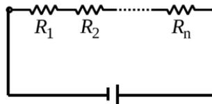
Figure 11 Connecting resistors in series.
