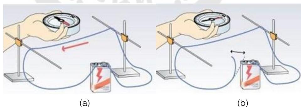
Figure 6 Shows experiment of Hans Christian Oersted (a) When an electric current and
