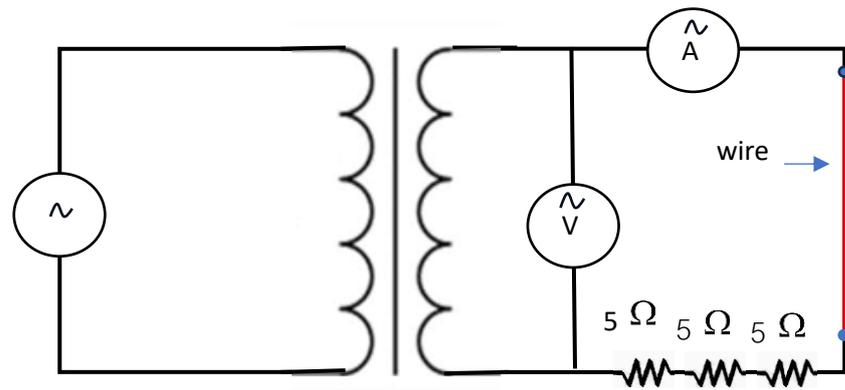
Figure 22 An electrical circuit such as 3 resistors connected in series.
