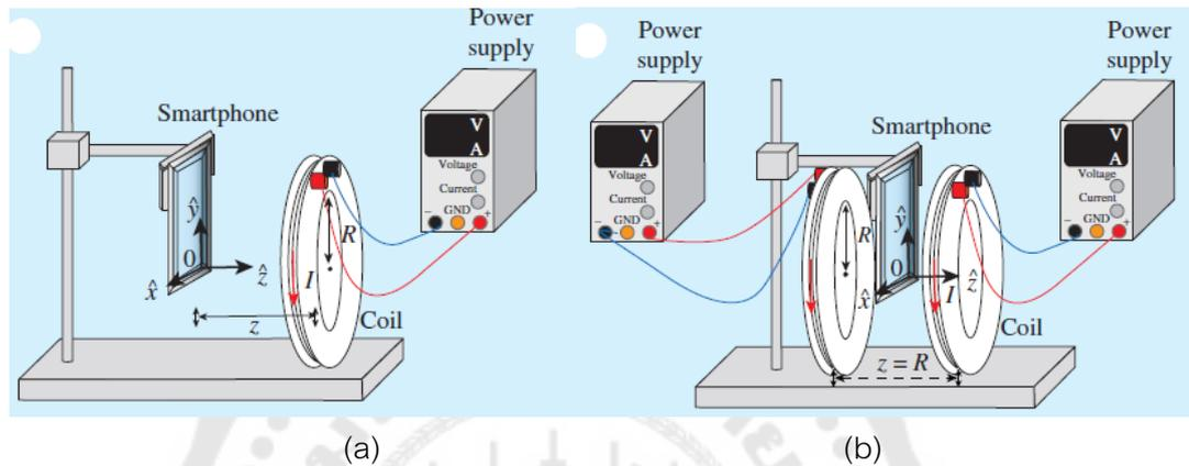
Figure 14 Measurement configuration of the magnetic field due to (a) one coil and (b) two coils.
