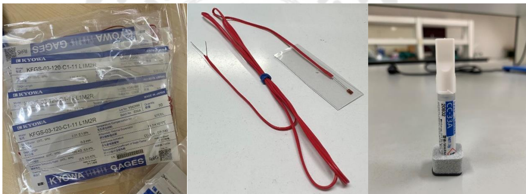
Figure 23 Strain gauge (Kyowa Electronic Instruments Co., Tokyo, Japan) and Cyanoacrylate-based cement (Strain Gage Cement CC—33 A-Kyowa Electronic Instruments Co., Tokyo, Japan).
