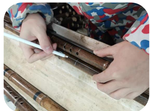
Figure75 Corrected hole space
