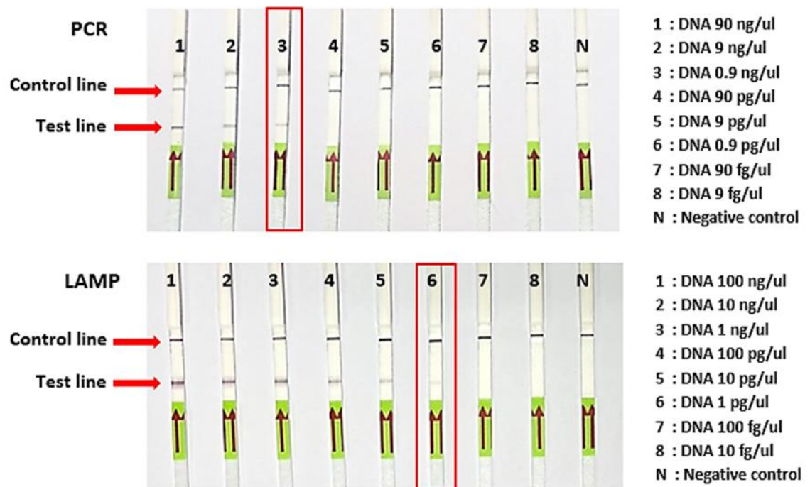
Figure 16 The LOD of PCR-LFD and LAMP-LFD assays. (PCR-LFD) Strips 1-8 represents amplification product of DNA concentrations at 90.0 ng/ \mu L, 9.0 ng/ \mu L, 0.9 ng/ \mu L, 90.0 pg/ \mu L, 9.0 pg/ \mu L, 0.9 pg/ \mu L, 90.0 fg/ \mu L, and 9.0 fg/ \mu L, respectively. (LAMP-LFD) Strips 1-8 represents amplification product of DNA concentrations at 100.0 ng/ \mu L, 10.0 ng/ \mu L, 1.0 ng/ \mu L, 100.0 pg/ \mu L, 10.0 pg/ \mu L, 1.0 pg/ \mu L, 100.0 fg/ \mu L and 10.0 fg/ \mu L, respectively. Lane N represents the negative control.
