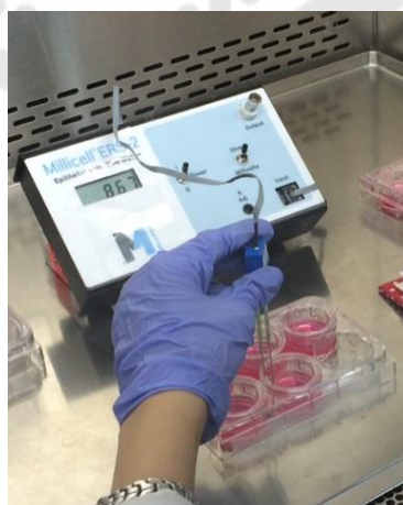
Figure 6 Measuring transepithelial electrical resistance across Caco-2 cell monolayer by volt-ohmmeter
