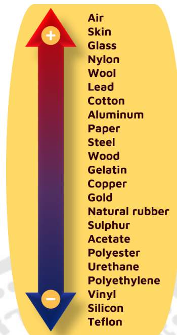
Figure 17 A triboelectric series of materials (51)
