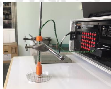
Figure 42 The example of measurement on cervical specimens with Clementine EIT.
