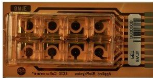
Figure 13 Specialized 8-well ECIS device. (3)
