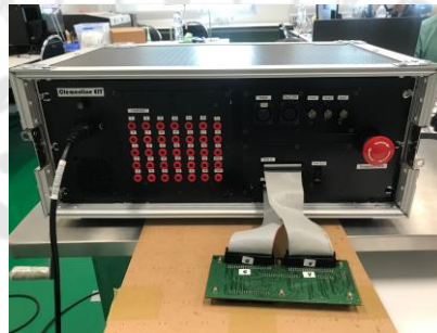
Figure 34 The resistor phantom connected to the machine.
