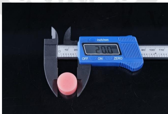
Figure 2 – Cylinder-shape milled acrylic resin, which was attached to pressure sensitive shaft of universal testing machine to detect compressive and tensile force, has a diameter of 20.0 \pm 0.5 mm.
