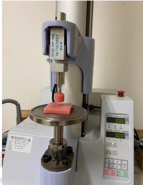
Figure 11 – Place sample holder in the center of the pressure sensitive shaft.
