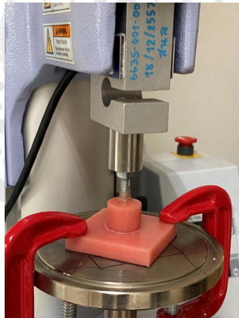
Figure 14 – The sample/sample holder assembly was placed on the adhesion test instrument's sample stand, with the load applied to the sample's center up to 10.0 \pm 0.2 N at a cross-head speed of 5 mm/min.
