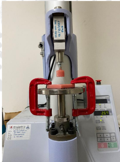
Figure 12 – Two of C-clamps were used to fix sample holder in the correct place.
