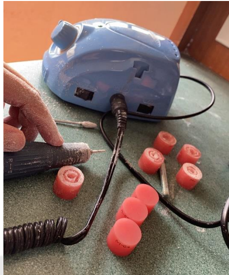
Figure 9 – Made a hold in the cylinder-shape PMMA, preparing cylinder-shape PMMA for pressure sensitive shaft holding screw attachment.
