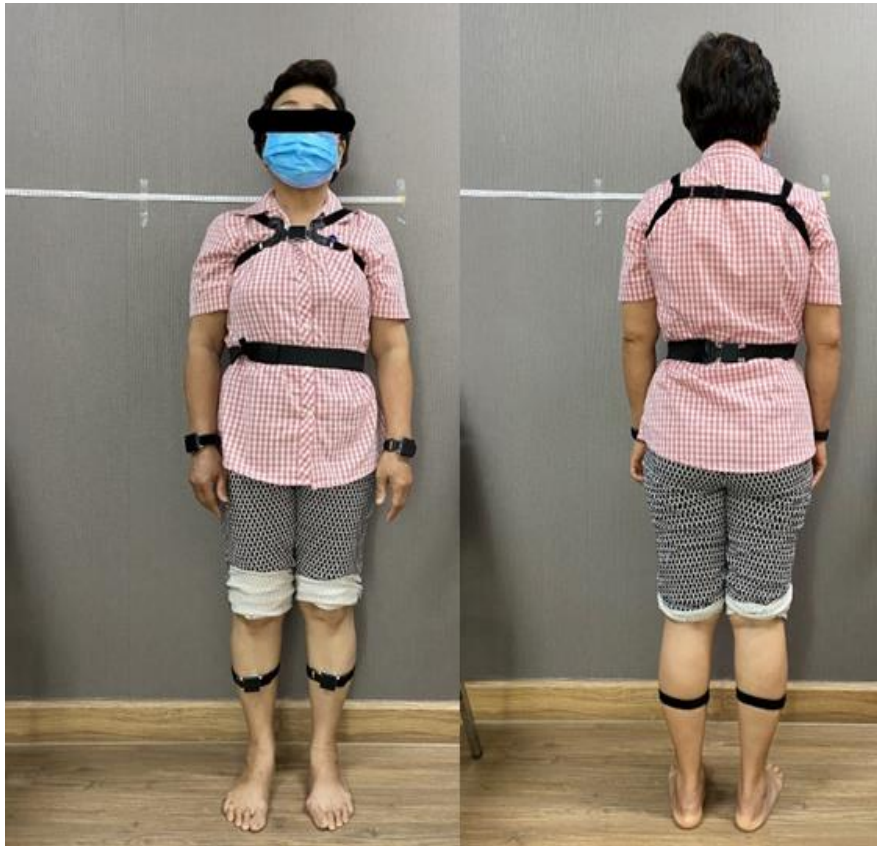
Figure 2 Wearable inertial sensors placement on the body
