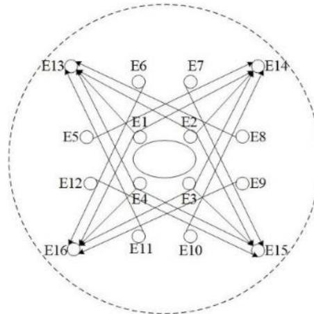
Figure 22 Planar electrode with the star layout.
