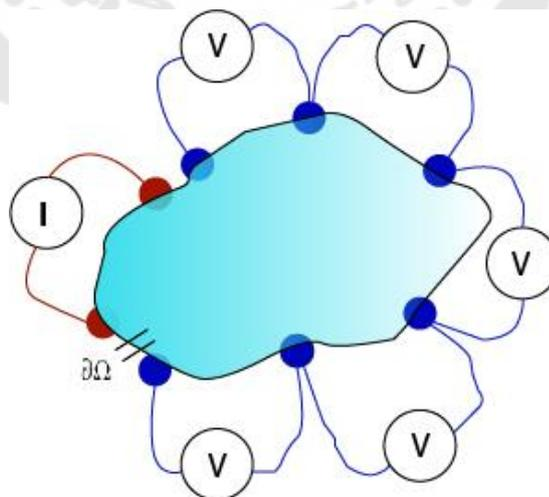
Figure 18 EIT system model on the boundary of the object under test. The constant electric current is injected through driving electrodes and the voltage information is measured with measurement electrodes.
