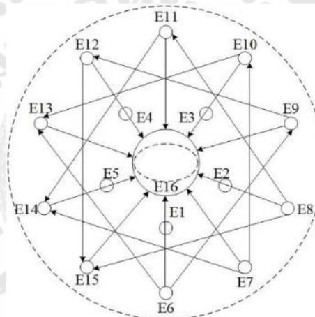
Figure 23 Planar electrode with the circular layout version 1.
