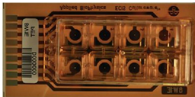
Figure 17 Specialized 8-well ECIS device. (The commercial model 8W1E PET)
